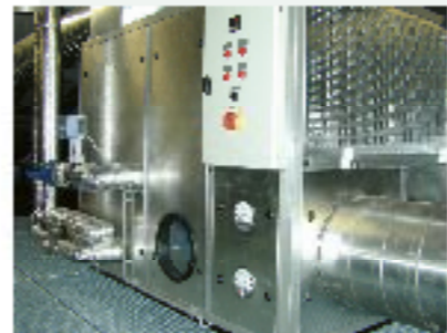
HYBRID, ABSORPTION & CONDENSATION INSTALLATION FOR DRYING & CONDITIONING Standard in any climate down to 5°C with 10% RH, specials also to -1-20°C and 20%RH
