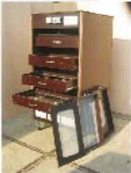
DRYER WITH DRAWERS AND TRAYS Drying of flower seed and small amounts of basic seed
