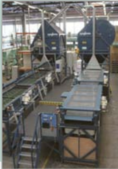
Flat screen sizers (5 fractions) with box tipple units
